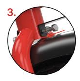
Put the fender bracket on the other end of the bolt.
