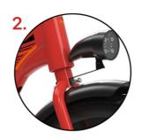
Insert the bolt and a washer into the headlight bracket, put the bolt through the hole in the fork.
