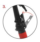
Close the buckle at the fold to fix the stem with your right hand
