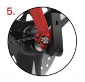
Fix the brackets on both sides of the fender and screw them tightly.
