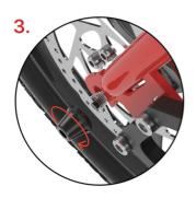
At the other end, put the spring first, the diameter inside small and the outside is large, and then put a nut
