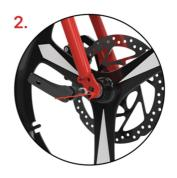
Insert into the hub from left to right, the quick release head is on the side without disc brake pads
