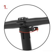
Loosen the quick release lever on the head of the stem
