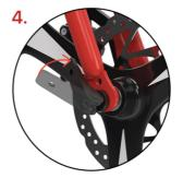
After adjusting both sides, close the quick release lever to lock
