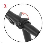
Lift the quick release lever on the handlebar, turn the handlebar to adjust the brake lever to the right position
