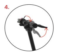
Finally, close the quick release lever on the handlebar to lock the handle bar.
