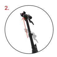
Lift the handlebar upward and height, then close the quick release lever
