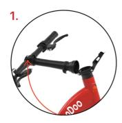
Hold the scooter frame and push up the folding stem to open it up.
