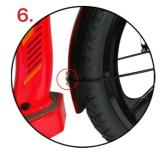
Adjust the clamp on the fender to make fender and brackets in right position.
